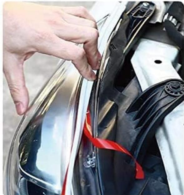
**Step 3:** Determine which daytime running lamp ACC connection comes first. Ensure 12V voltage, with a current of 10A, and take care not to cut any wires.
